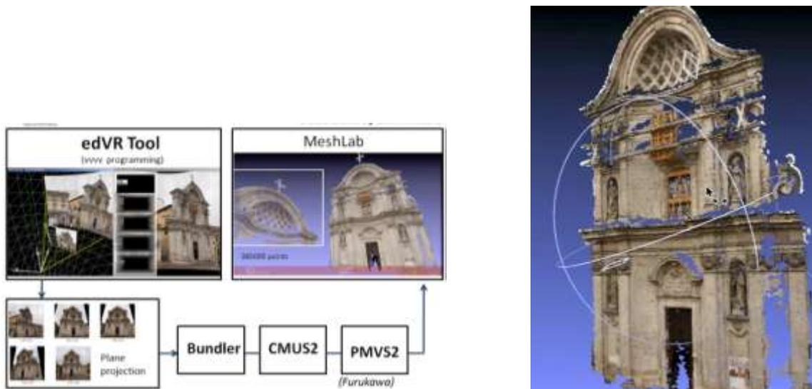
Figure 5 – The flow-chart of the elaboration of the panorama to get the point cloud with Structure from Motion approach with PMSV2 by Furukawa and Ponce
