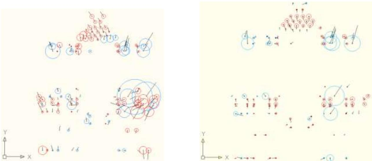
Figures 8 and 9 – The errors distribution (amplified x30) 28 mm focal length freehand held camera (left) and tripod in spherical head (right)
